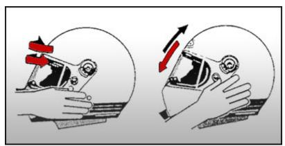
After you have made your visual check, grab the helmet in your hands - one on either side - and try to rotate the helmet from side-to-side. Note any movement of the skin while doing this, as well as the amount of resistance to movement. Hold your head steady to do this.
